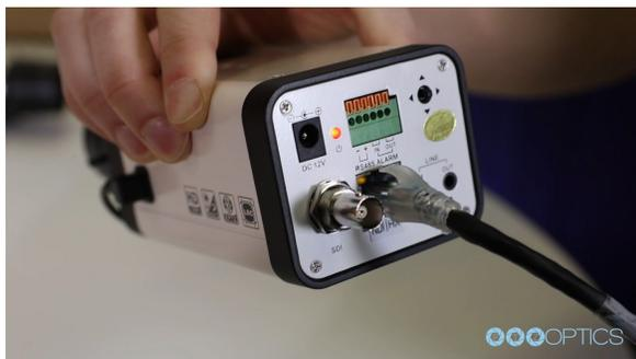
**Step 4:** Once you have selected a method of powering your camera, you can plug it in and the camera will turn on automatically. You will see the power light illuminate once the camera has successfully powered on.
