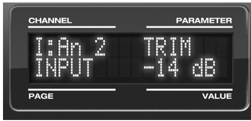
Figure 4-6: Setting the input trim for a TRS analog input pair.
