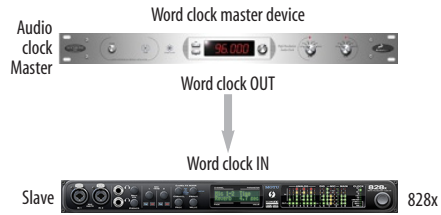
Figure 4-18: Slaving the 828x to word clock. For the 828x clock source, choose 'Word Clock In'.
