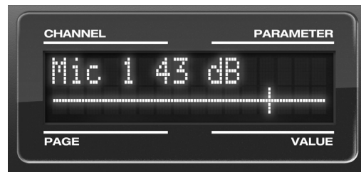
Figure 4-3: The LCD gives you feedback as you turn the TRIM knobs for the two mic/guitar inputs.
