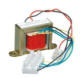
The T20 is an 8 ohms to 100 volt transformer. By using the T20 you can change a standard 8 ohms loudspeaker into a 100 volt loudspeaker.
