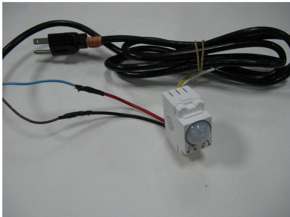
(2) Connect motion sensor to IAdea GPIO extender, in this setup, IN0 port is used.
