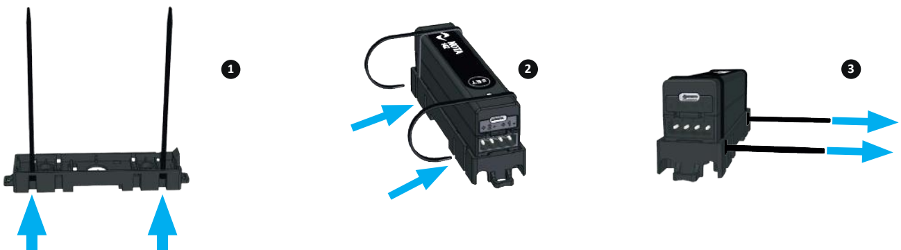
Figure 6 – Cable ties secure attachment amplifier-support
