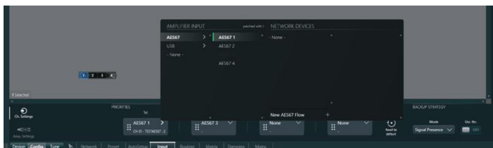
Figure 16- Input patching panel on ArmoníaPlus
