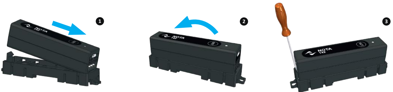
Figure 5 – Mounting on support add-on
