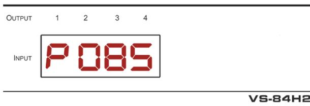
In this example: Input 8 is routed to output 3, input 5 is routed to output 4, a pattern is routed to output 1, and output 2 is set to mute.
