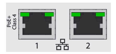
Connect network port 1 to a PoE+ switch to enable quick recovery of audio when the mains supply is temporarily lost. Audio from the device, including from the analog inputs, is not available while the device is powered from PoE+. Powering the device requires a compliant PoE+ class power source or above.
