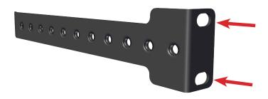
3. Screw the M6 mounting screw into the appropriate hole for both rear support brackets. Leave enough room between the head of the screw and rear bracket for the slotted end of the mounting brackets.
