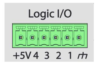
These Logic I/O connections can be used as either inputs or outputs. They can be assigned to actions within Tesira software using Logic Input and Logic Output.
