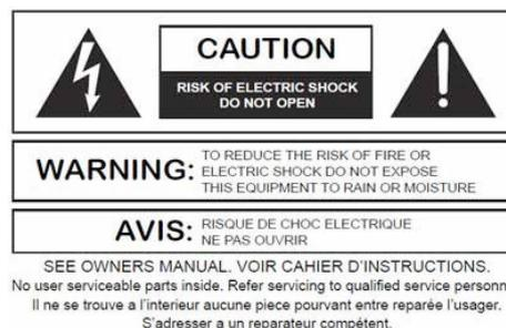
The lightning logo (an equilateral triangle with an arrow) is used to make the users aware of the uninsulated "dangerous voltage" within the product shell, which may cause electric shock. An equilateral triangle with an exclamation mark is adopted to make the users understand the importance of the operations and maintenance instructions given in the appendixes attached to the product.
