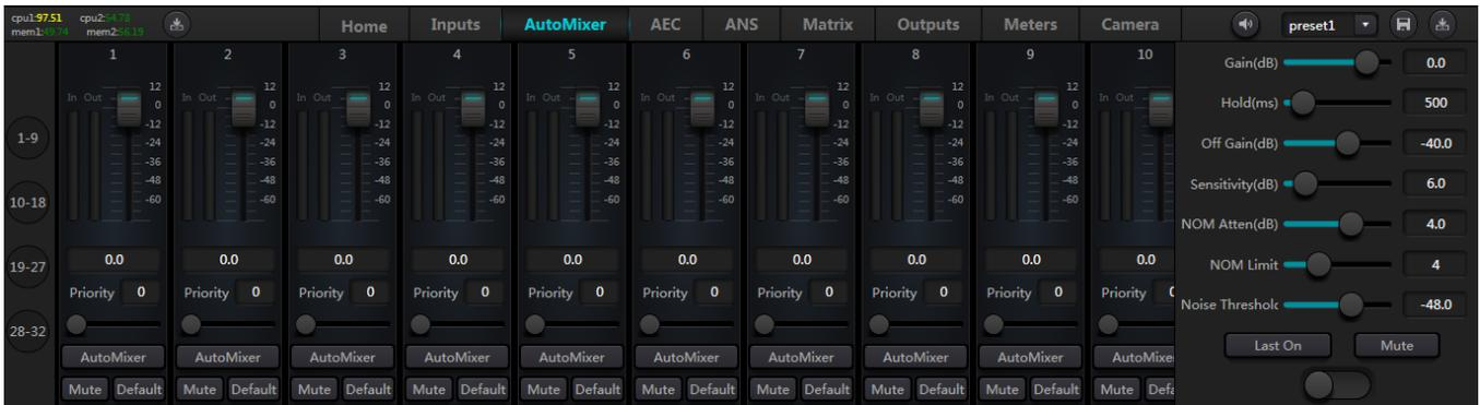
The threshold automatic mixer is based on the noise gate development, each channel has a noise gate, which is either open or closed.
