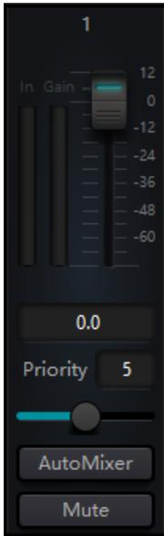
**Auto Mix:** Each channel has an automix on/off button which must be turned on for channels need to participate in automix. It may also be closed, and then the channel will not participate in automix.
