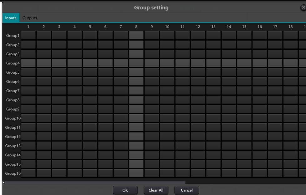
Each group can select 1- the maximum number of channels for the device. The maximum number of channels for the device depends on the model you purchased. The channel is set as a group, which will be distinguished by a color on the Home screen.
