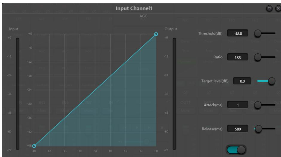
Auto gain control includes the following control parameters and switches:
