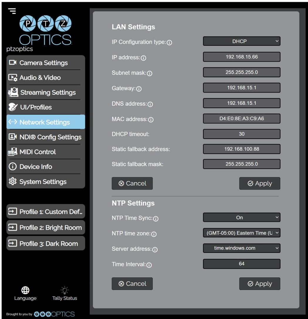
The screenshot displays the Network Settings page within the PTZ OPTICS application. The interface is divided into a left sidebar and a main content area.
