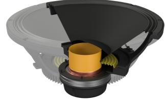
The unique SilentFlow laminar flow port technology of our proprietary phase inverter minimizes air noise at high output levels by reducing turbulence, plus increases its lowfrequency efficiency.
