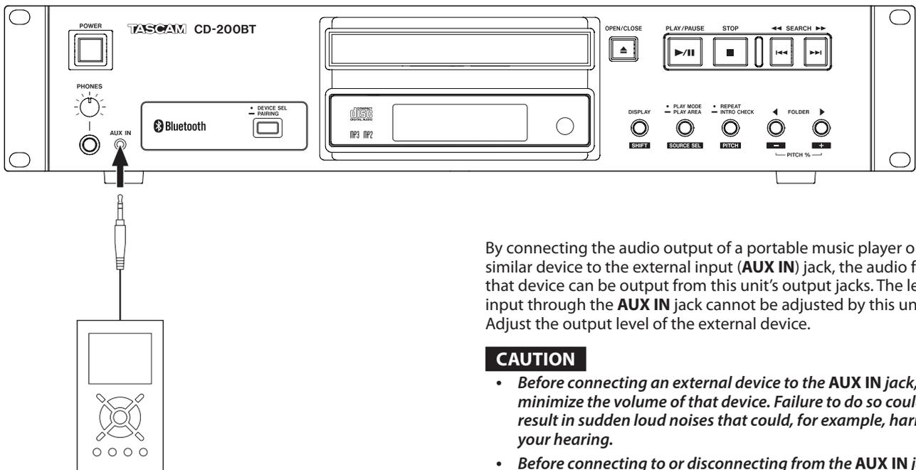
By connecting the audio output of a portable music player or similar device to the external input (**AUX IN**) jack, the audio from that device can be output from this unit's output jacks. The level input through the **AUX IN** jack cannot be adjusted by this unit. Adjust the output level of the external device.
