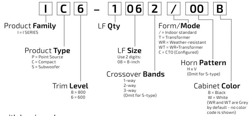
The standard configuration is indoor construction with low impedance operation. All models also have T, WR and WT versions
