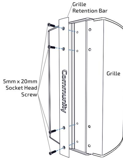
**Figure 3a.** Remove one retention bar, loosen that side of the grille and then remove the other retention bar
