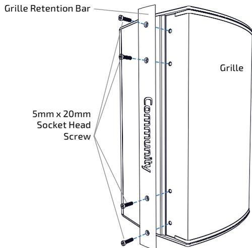
Figure 6a. Remove one retention bar, loosen that side of the grille and then remove the other retention bar
