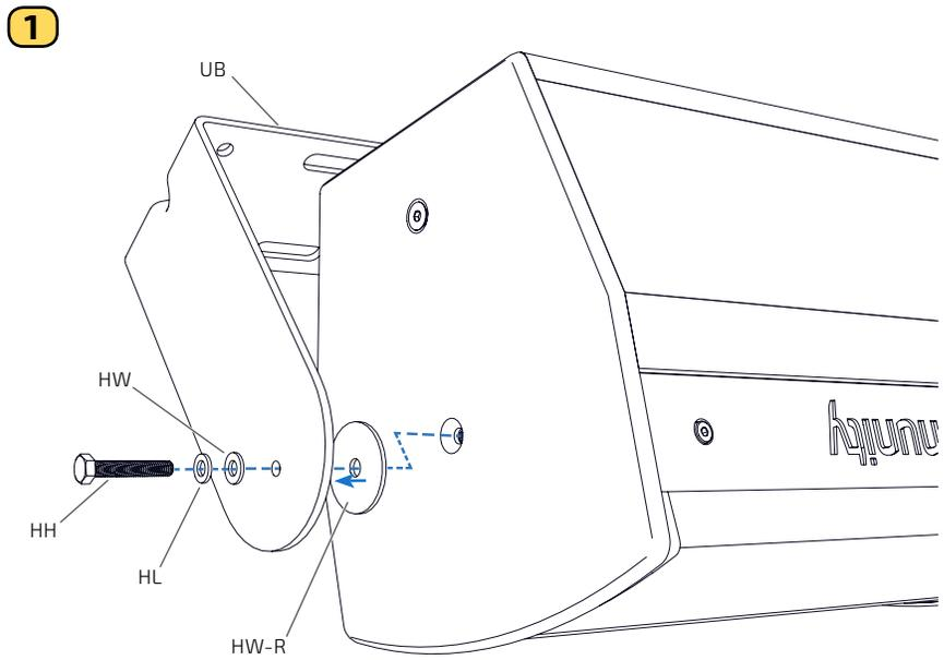
**Figure 1.** Remove middle cabinet bolts and attach yoke to cabinet
