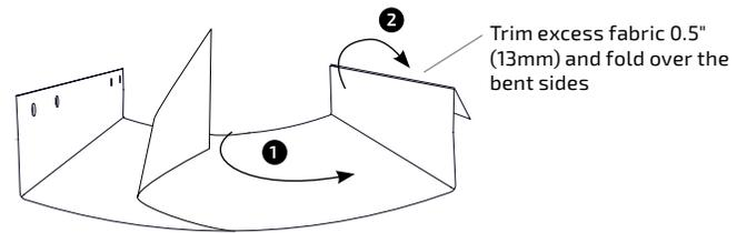
**Figure 7b.** Press fabric against grille and into the bends, smoothing out any wrinkles
