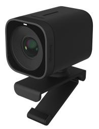
The Vidi<sup>™</sup> 250 is a wide angle 4k camera designed for use with conferencing systems. Intended for huddle rooms or small to medium conferencing rooms, the Vidi 250 has a 120° field of view, allowing everyone in the room to be seen. The Vidi 250 uses auto framing technology to adjust the focus and zoom to keep participants in view. The Vidi 250 can be either display mounted or wall mounted.
