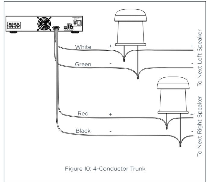
Figure 10: 4-Conductor Trunk
