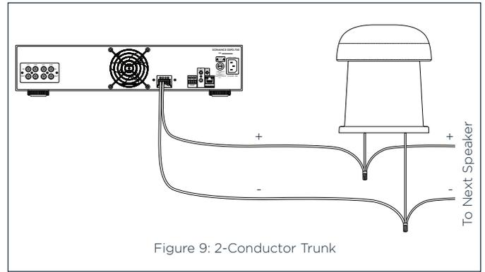
Figure 9: 2-Conductor Trunk
