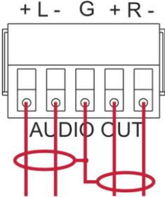
Figure 4: Connecting to a Balanced Stereo Audio Acceptor
