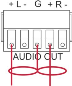
Figure 5: Connecting to an Unbalanced Stereo Audio Acceptor
