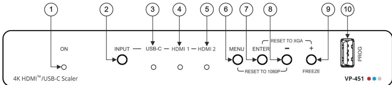
Figure 1: VP-451 HDMI / USB-C Scaler Front Panel
