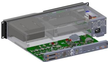
5. Inspect the CAT1700 main board for signs of damage to its components or the edge connector that plugs into the CAT1720 front panel. If there is damage, you may need to replace the CAT1700 or CAT1720.
