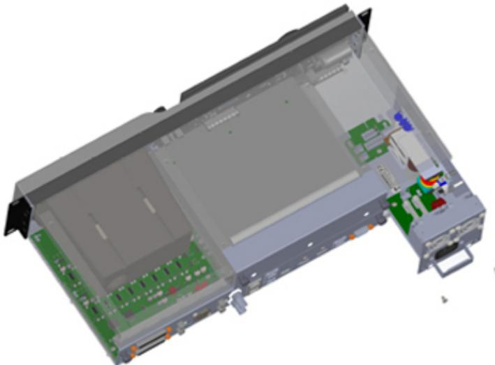
8. Detach the DC power cables (both plugs) from the CAT1741 power supply assembly.
