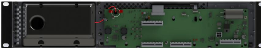
19. If you are experiencing a problem with the front-panel touch screen, check and reseal the two small ribbon cables at the top of the circuit board (gold colored ribbons).
