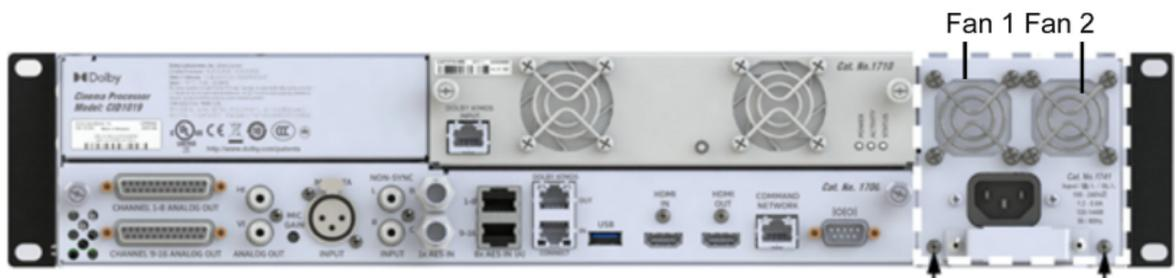
5. Use a small Phillips screwdriver to remove the two screws that secure the power supply to the chassis.
