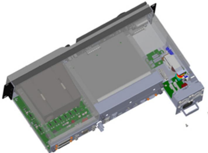
7. **Warning:** The power supply may retain high voltage after removing. Wait at least 15 minutes before touching power supply components after removing.
