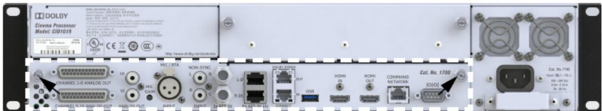
3. Unscrew the thumbscrews in a counter-clockwise direction. These screws are locked into the board chassis and do not come out completely.
