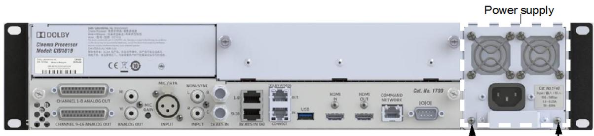
3. Use a small Phillips screwdriver to remove the two screws that secure the power supply to the CP950 chassis.
