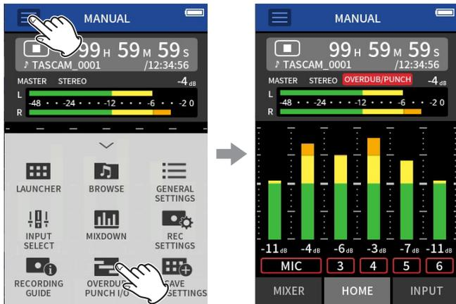
3. Open the INPUT screen, and ready the tracks to be recorded (red).
