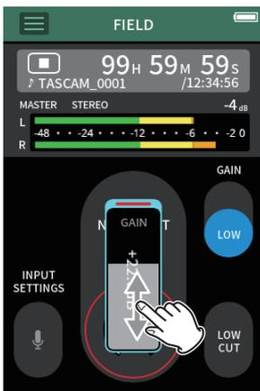
While pointing the mic at the recording subject and watching the level meter, adjust the GAIN so that the level averages around  $-12$  dB and the PEAK indicator does not light.
