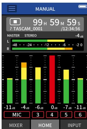
When it appears like this, the input is overloading and the sound could be distorted. If this occurs, make adjustments in the following ways so that the sound does not distort.
