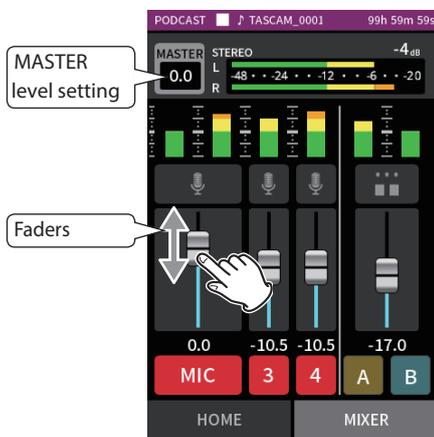
Each project will play back with the mix balance used when it was recorded. Changes to a mix balance during playback will not be saved. Use the mixdown function to change the mix balance of a project that has already been recorded. (see "Mix down function" on page 71)
