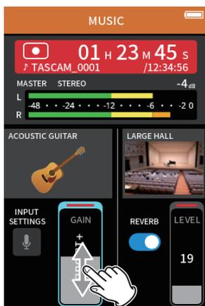
While playing an instrument and watching the level meter, adjust the GAIN so that the level averages around  $-12$  dB and the PEAK indicator does not light.
