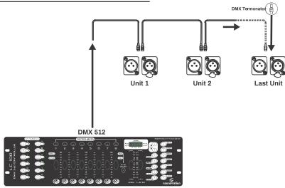
Connect the DMX output of the first fixture in the DMX chain with the DMX input of the next fixture. Always connect one output with the input of the next fixture until all fixtures are connected.
