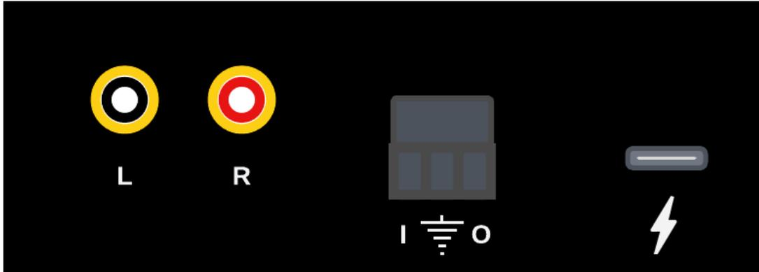
! The current firmware only supports a single audio channel. Only the LEFT channel input will be used.
