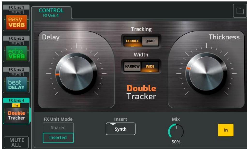
**FX Unit Mode** – ‘Shared’ allows multiple channels to send signal to the FX Unit simultaneously, and for the output of the FX Unit to be sent to Main LR, Outputs or other FX Units at different levels from either the PROCESSING / SENDS screen, or in the FADER screen. Shared mode is generally used for reverbs and delays. ‘Inserted’ allows the FX Unit to be used in a single input or output channel, to use a Chorus on a violin for example.
