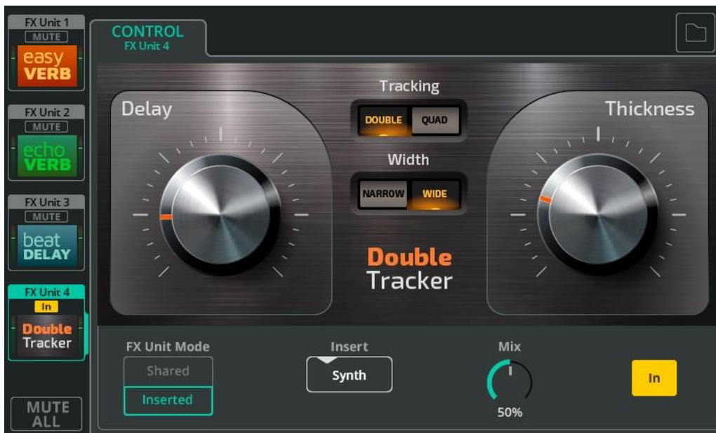
The Double Tracker recreates the classic studio effect of recording (or ‘tracking’) the same source multiple times, where slight differences in each recording result in a bigger, thicker sound.
