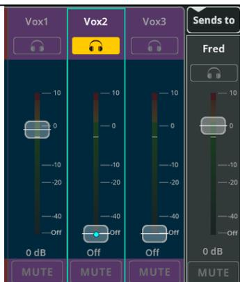
3. Raise the fader for any Input in order to send signal from that input channel to the selected Output.
