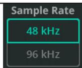
3. Select the **Sample Rate**. 48kHz allows for longer recording time and more channels to be recorded at a lower quality. 96kHz allows a maximum of 16 channels to be recorded for a shorter time but at the highest quality.
