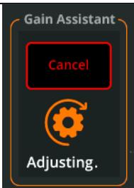
6. Make noise into the connected microphone or with the connected instrument/source to let the Gain Assistant know what the typical signal level will be.
