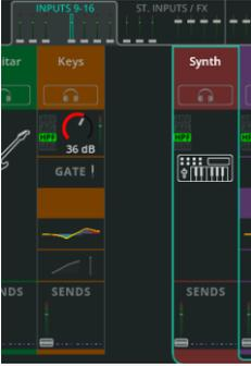
1. Go to **PROCESSING**, locate the bank of faders from the top of the screen containing the channel with processing to be stored.
