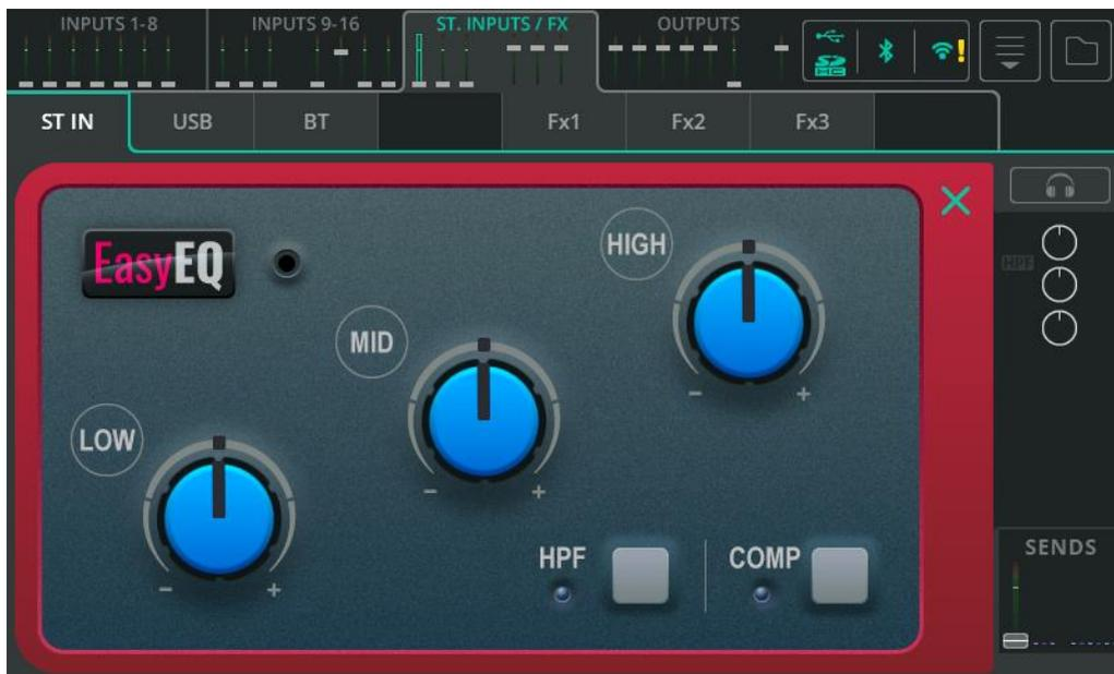
The EasyEQ is a unique Quick Channel which is in fact a model of the MusiQ found in the Allen & Heath ZED range of analogue mixers, with the added benefit of a compressor.
