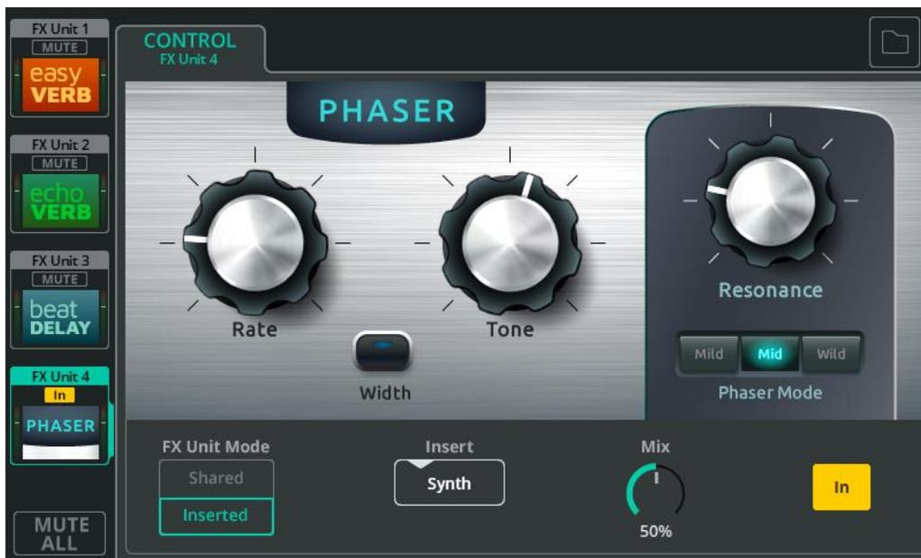
The Phaser combines the original signal and a copy of the signal with phase shifting applied at different frequencies. This causes some frequencies to cancel out at the same time as others are reinforced.
