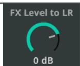
6. Set the **FX Level to LR** to 0dB as a starting point. This controls the amount of 'wet' FX signal being heard in the Main LR.
