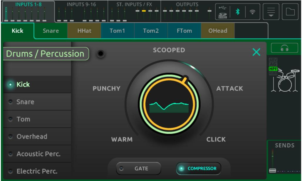
A 'one knob' Quick Channel has instrument or source types on the left-hand side. Select one of the options on the left, then touch the large main dial and use the touchscreen rotary (CQ-12T, CQ-18T) or touch and drag (CQ-MixPad) to adjust to taste.
