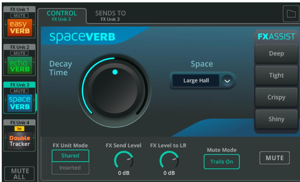
Space Verb includes various reverberant spaces and classic plate reverbs, it's designed to help unify a mix by putting multiple inputs into the same virtual space.
