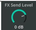
5. Set the **FX Send Level** to 0dB as a starting point. This can be adjusted at any time to control the overall signal level being fed into the FX Unit.
