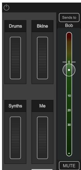
The main screen displays the overall output level on the right, with the ability to select the output being controlled above this, and a mute at the bottom.
