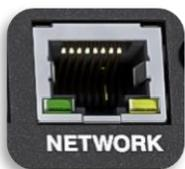
RJ45, Fast Ethernet. For network control messaging only.
