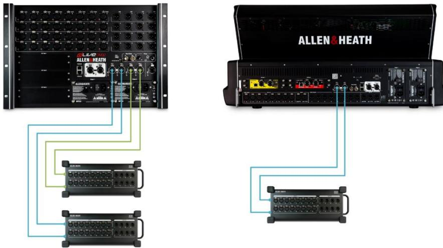
**dLive C Class Surfaces, C Class MixRacks and Avantis** mixers can benefit from DX redundancy via the use of DX Link and/or DX Hub options.
