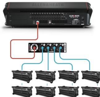
Up to 2x DX Link I/O modules, or gigACE+DX Hub combinations, can be installed in the I/O ports to further expand DX connectivity up to a maximum of 24x DX Expanders
