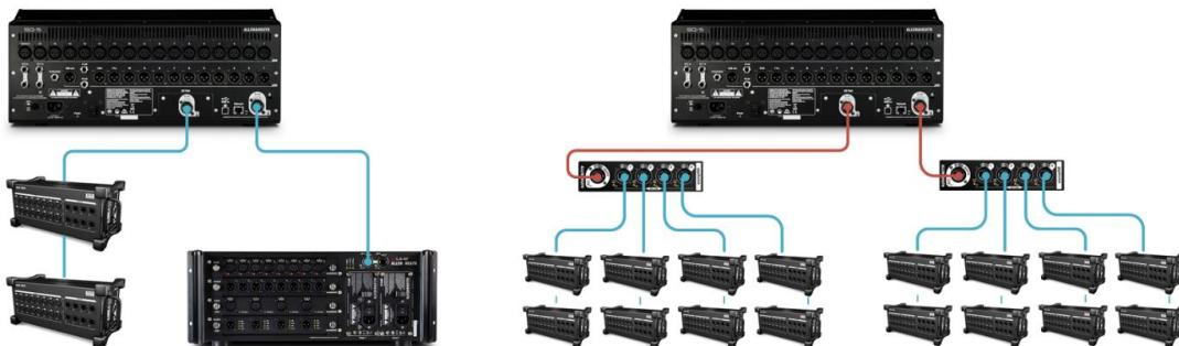
① SQ does not support DX redundancy
