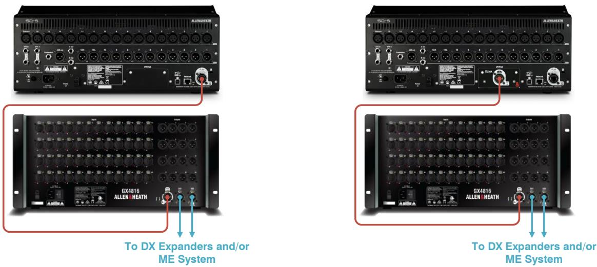
The connection of 2x GX4816s is supported via the use of both the internal SLink port and the optional SLink I/O module.
