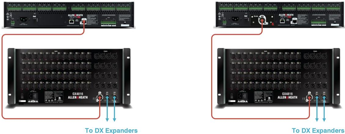
The connection of 2x GX4816s is supported on AHM-64 via the use of both the internal SLink port and the optional SLink I/O module.
