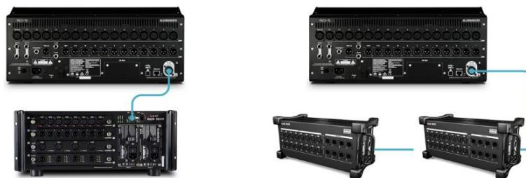
Alternatively, a DX Hub can be connected to the SLink port to provide 4x DX connections enabling the use of up to 8 DX expanders.
