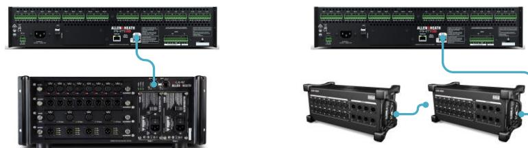
Alternatively, a DX Hub can be connected to the SLink port to provide 4x DX connections enabling the use of up to 8 DX expanders.
