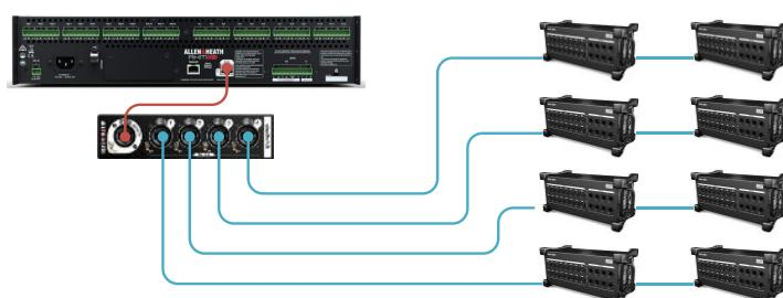
An optional SLink I/O module can be installed in the AHM I/O port to enable further DX connectivity.
