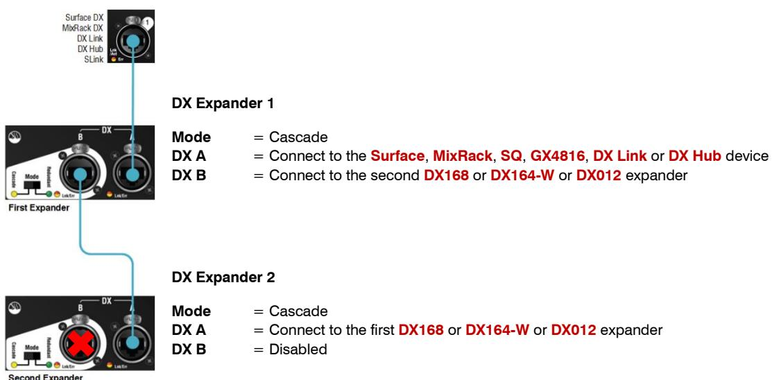
Please refer to the table below for channel mapping when using DX Expanders in Cascade mode.
