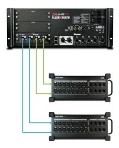
Two DX Hub units can be used to achieve DX redundancy for up to 4 DX expanders. Both DX Hub units connect to a single gigaACE I/O module in a dLive or Avantis system:
