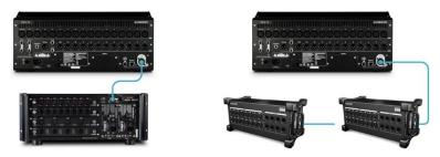
Alternatively, a DX Hub can be connected to the SLink port to provide 4x DX connections enabling the use of up to 8 DX expanders.
