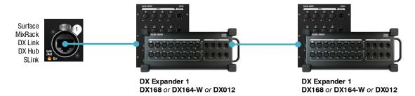
Any combination of two DX168/DX164-W/DX012 expanders is supported per socket in Cascade mode, with all inputs and outputs accessible to the mix engine.
