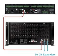
The connection of 2x GX4816s is supported on AHM-64 via the use of both the internal SLink port and the optional SLink I/O module.
