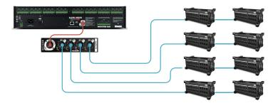
An optional SLink I/O module can be installed in the AHM I/O port to enable further DX connectivity.
