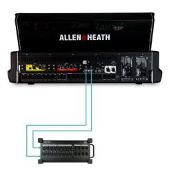
dLive C Class Surfaces, C Class MixRacks and Avantis mixers can benefit from DX redundancy via the use of DX Link and/or DX Hub options.
