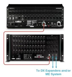
The connection of 2x GX4816s is supported via the use of both the internal SLink port and the optional SLink I/O module.
