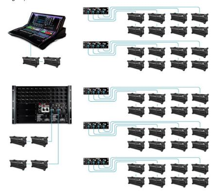
A fully expanded C Class system with 2x DX Hub/DX Link and 22x DX168 would add 352 inputs and 176 outputs to the system (DX Link shown in diagram)
