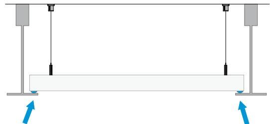
Installing the TeamConnect Ceiling 2 in the ceiling without angle brackets (600 x 600 mm grid)
